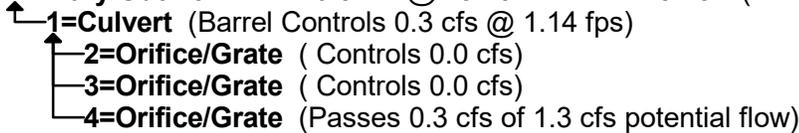
**Secondary OutFlow** Max=0.3 cfs @ 15.19 hrs HW=25.78' (Free Discharge)
