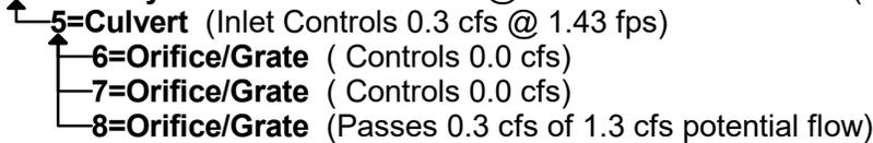
**Tertiary OutFlow** Max=0.0 cfs @ 0.01 hrs HW=25.50' (Free Discharge)
